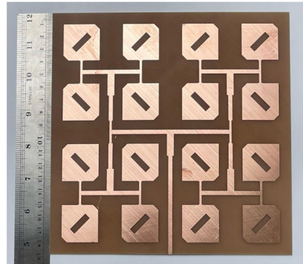
Fig. 5. Fabricated microstrip antenna.
