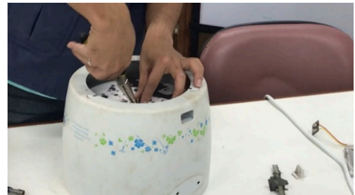
Fig. 16. Disassembly tasks of the electric rice cooker.
