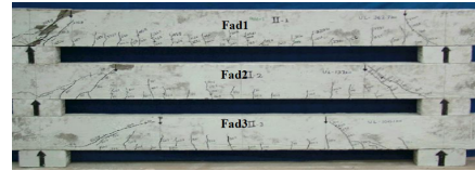
Fig. 8. Photographs of tested beams for Series-F.
