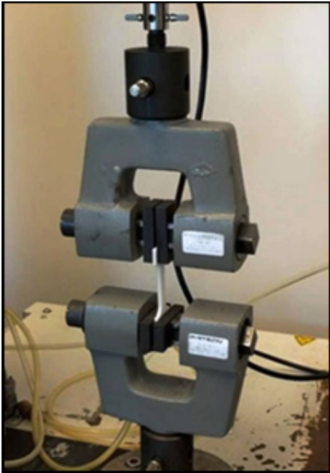
Fig. 3. Experimental set-up for tensile testing.
