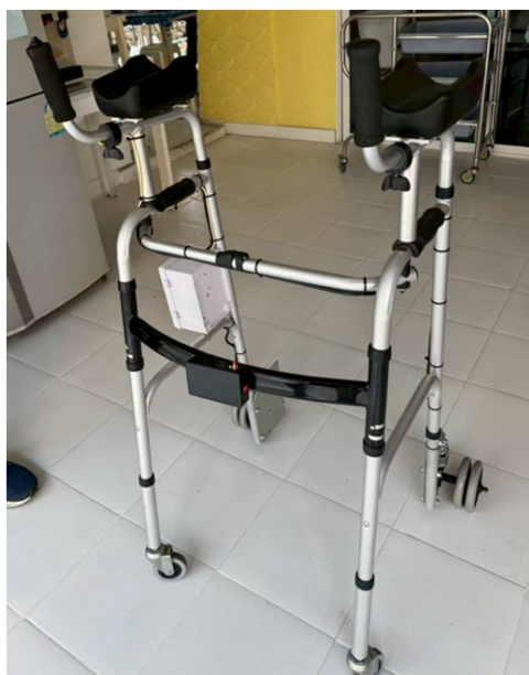
Fig. 1. Prototype of the motorized smart walker used in this study.
