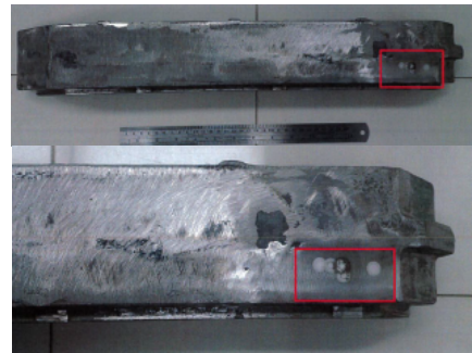
Fig. 9. Overall photograph of the Grate bar using the optical emission spectrometer (OES) test method.
