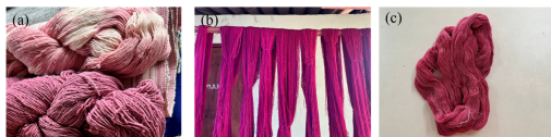
Fig. 2. Images of yarn dyed using the (a) pre-improvement method and (b, c) post-improvement method, demonstrating enhanced color uniformity and consistency after process refinement.
