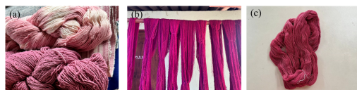
Fig. 2. Images of yarn dyed using the (a) pre-improvement method and (b, c) post-improvement method, demonstrating enhanced color uniformity and consistency after process refinement.
