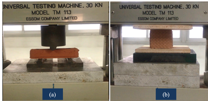
Fig. 6. (a) Flexural strength test and (b) Compressive strength test.
