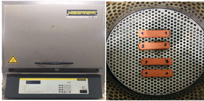
Fig. 5. 3D-printed clay specimens subjected to the sintering process.
