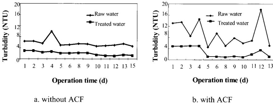
**Figure 3** Variation of turbidity in effluent in SSF
