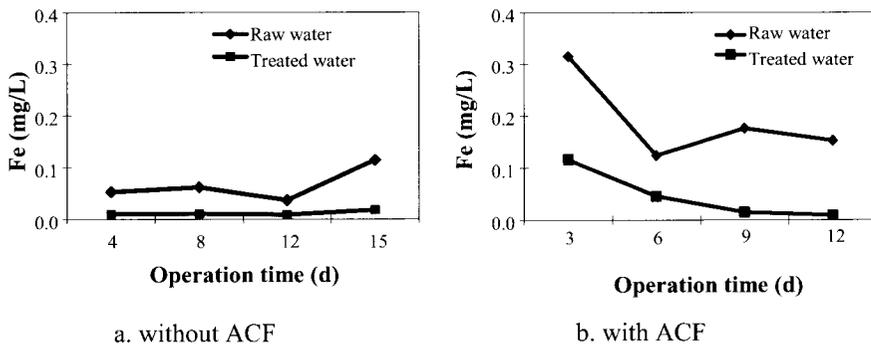
Figure 4 Variation of iron in effluent
