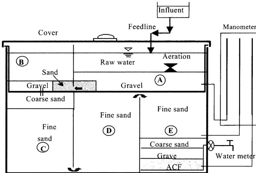
**Figure 1** Schematic diagram of the household water filter
