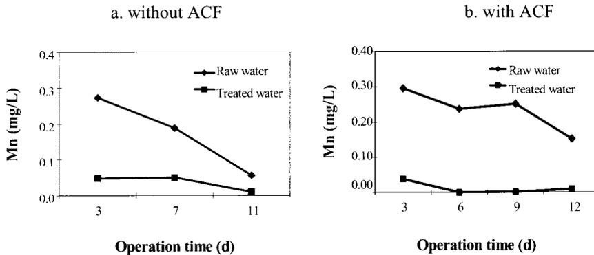
Figure 5 Variation of manganese in effluent
