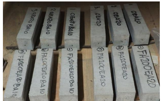
4a) Specimens for free expansion/shrinkage test
