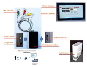
**Figure 2.** The W&C EKG components recorded and displayed the EKG signal via WD mycloud.
