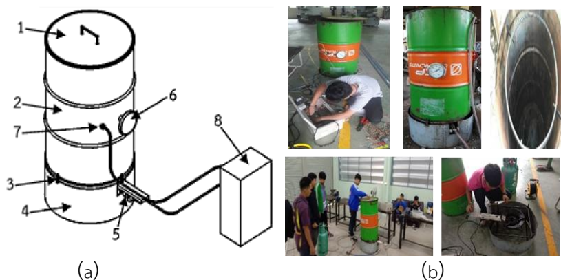
Figure 1 (a) Work design (b) Prototype of a low-cost heating oven based on the Sufficiency Economy
