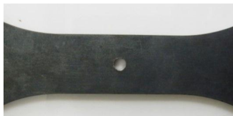
Figure 5 Original surface color of fatigue test specimen before grinding.
