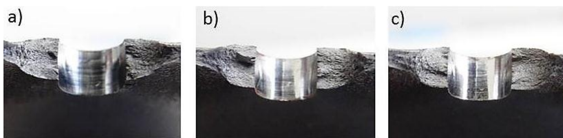
Figure 9 Fracture surface of a) SD, b) SNC and c) ENC fatigue specimen tested at stress amplitude of 123 MPa.
