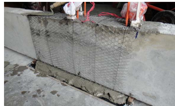
a) Strengthening of specimen by ferrocement
