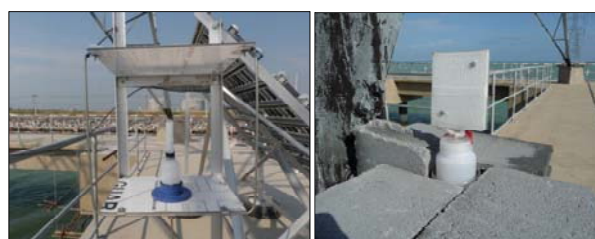
Fig.3 The wet candle installed on the rack No.2 (left) and the wet plate installed at the leg of transmission tower (right)
