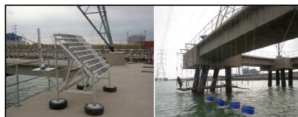
Fig.2 The exposure rack of atmospheric zone (left) and tidal zone (right)
