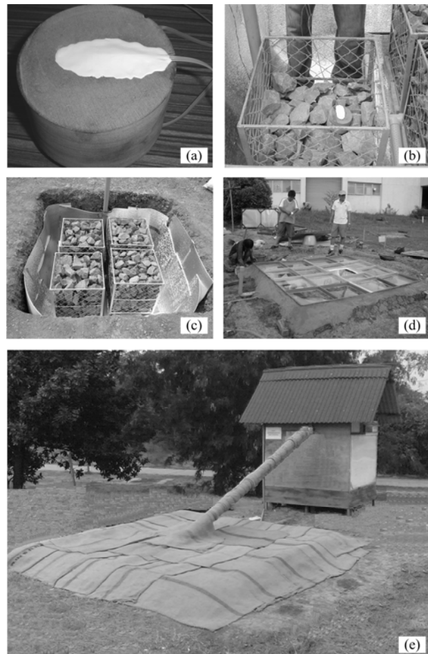
Figure 4 Scaled-down model for solar thermal energy storage. (a) thermocouple attached in surface of rock fragment, (b) rock fragment with thermocouple is laid in rock basket, (c) baskets of rock fragment, (d) Acrylic sheet reinforced with steel frame, and (e) storage system connected to housing with tube.
