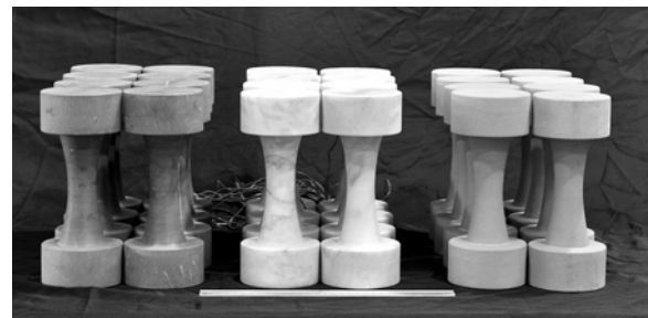
Figure 2 SB limestone (left), SB marble (middle) and PP sandstone (right) specimens prepared for direct tensile testing.
