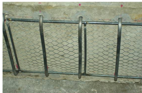
(a) C-shaped reinforcement (external web reinforcement)
