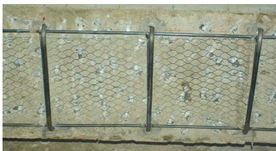
(a) Increasing the surface roughness for S200SR
