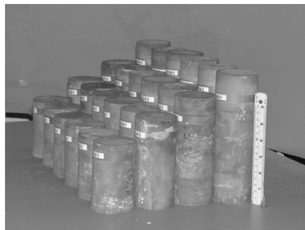
Figure 1. Some claystone specimens with L/D ratios of 1.5, 2.0, 2.5 and 3.0.
