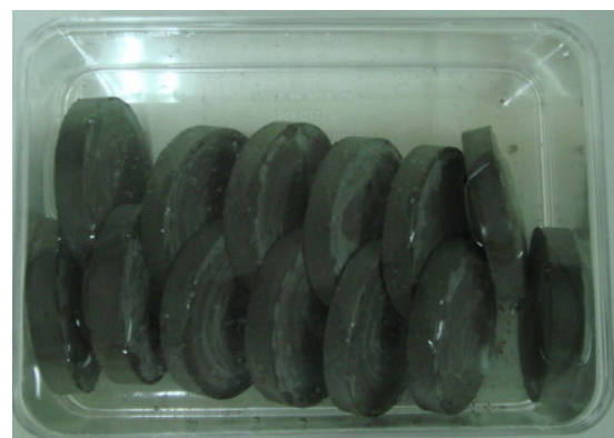
Figure 3 Paste specimens for chloride binding capacity and chloride penetration test
