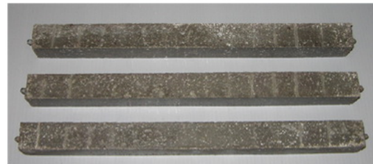
Figure 2 Mortar specimens using for sulphate resistance test
