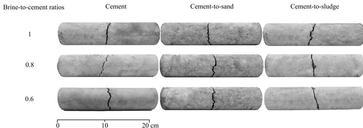
**Figure 4** Examples of post-test specimens from four-point bending test
