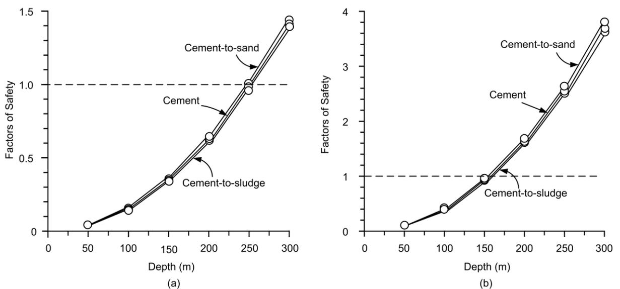
**Figure 7** Factors of safety as a function of depth calculated by tensile strain energy (a) and the Coulomb's criterion (b)
