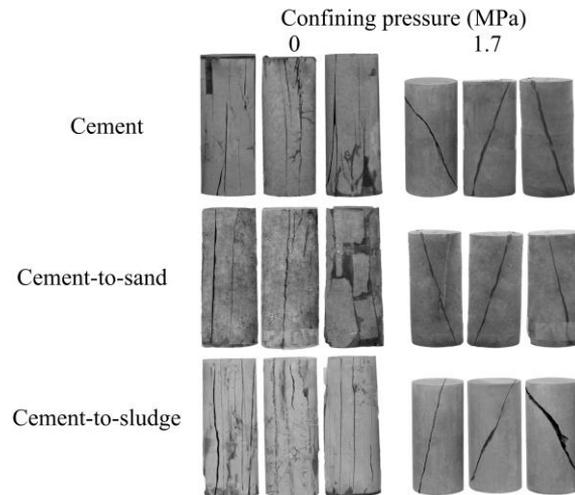
Figure 1 Examples of post-test specimens from uniaxial and triaxial compressive strength tests
