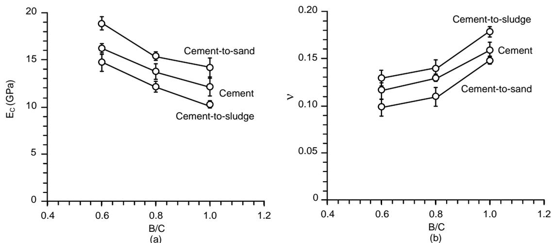
Figure 3 Elastic modulus ( $E_c$ ) (a) and Poisson's ratio ( $\nu$ ) (b) as a function of brine-to-cement ratio ( $B/C$ )
