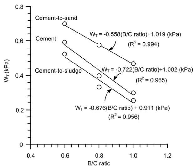
Figure 5 Total strain energy densities ( $W_T$ ) as a function of brine to cement ratios ( $B/C$ )
