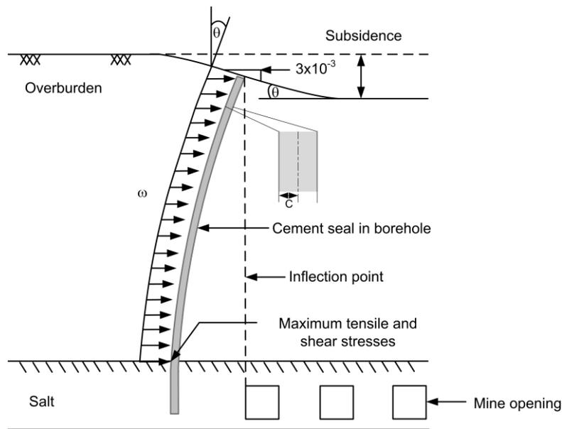
**Figure 6** Cement seal in borehole under bending with maximum ground surface slope of  $3 \times 10^{-3}$
