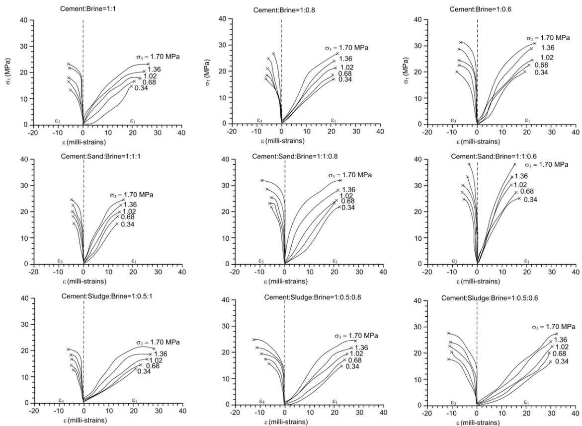
Figure 2 Stress-strain curves for compression tests
