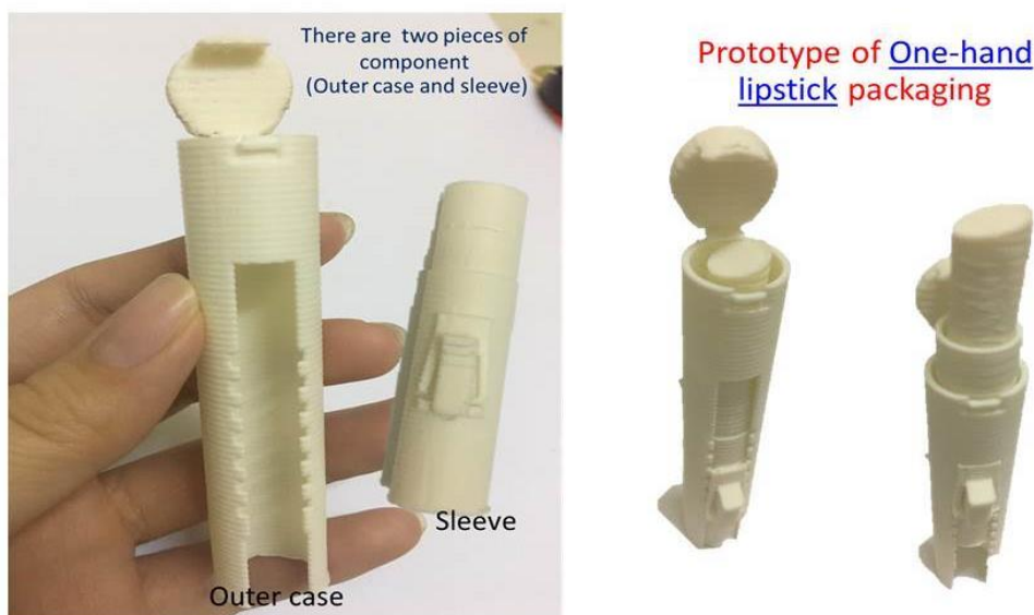
Figure 6 Prototype of One-hand lipstick packaging generated by 3-D printer (outer case and sleeve)
