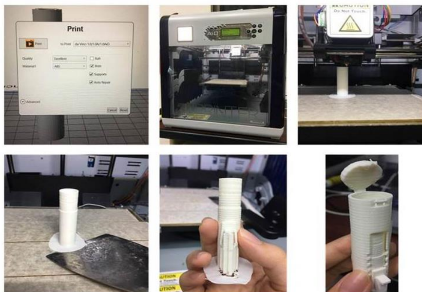
Figure 5 New design prototype generated using 3-D printing process
