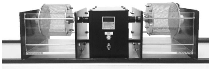
Figure 1 Slake durability test apparatus [1]
