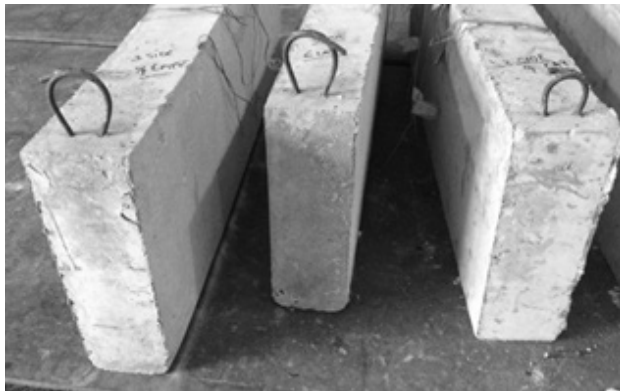
Figure 3 Rounded corners of U-wrapped specimens
