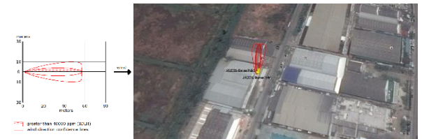
Fig. 8 Scenario6, wind speed: 12m/s, temperature: 37.5 °C, wind direction: South
