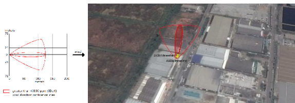
Fig. 5 Scenario3, wind speed: 2.6m/s, temperature: 37.5 °C, wind direction: South
