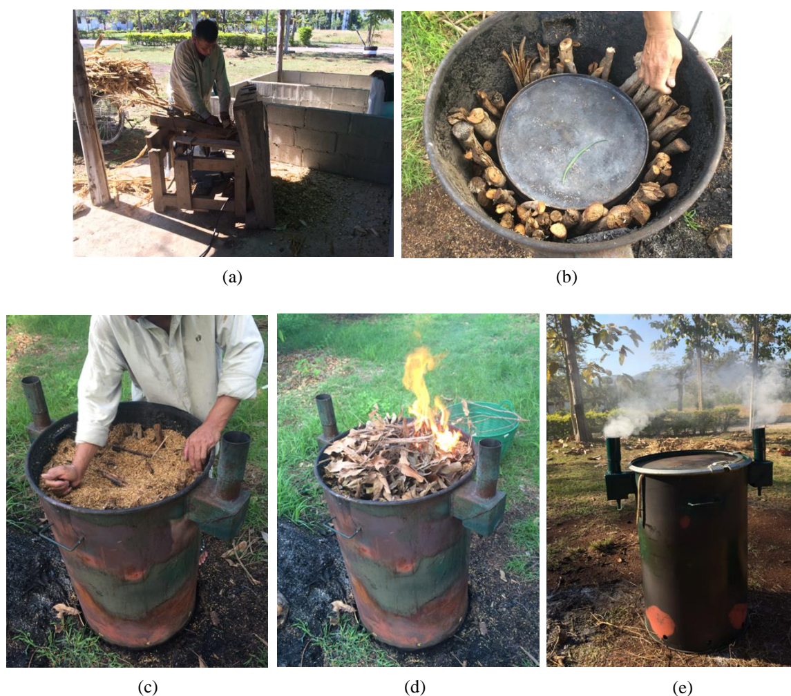
Figure 1. The various steps during the production of biochar from maize: a) Maize stalk chopping; b-c) Placement of firewood and rice husks in the outer burner tank; d) Biochar fire starter; e) Continuous combustion.
