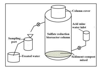
Figure 3. Schematic of the bioreactor for sulfate reduction
