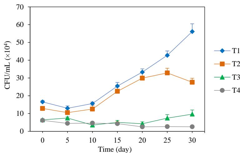
**Figure 6.** Number of sulfate-reducing bacteria in acid mine water with treatments: 10% sediment and 5% compost (T1), 10% sediment (T2), 5% compost (T3) and without added sediment and compost (T4).
