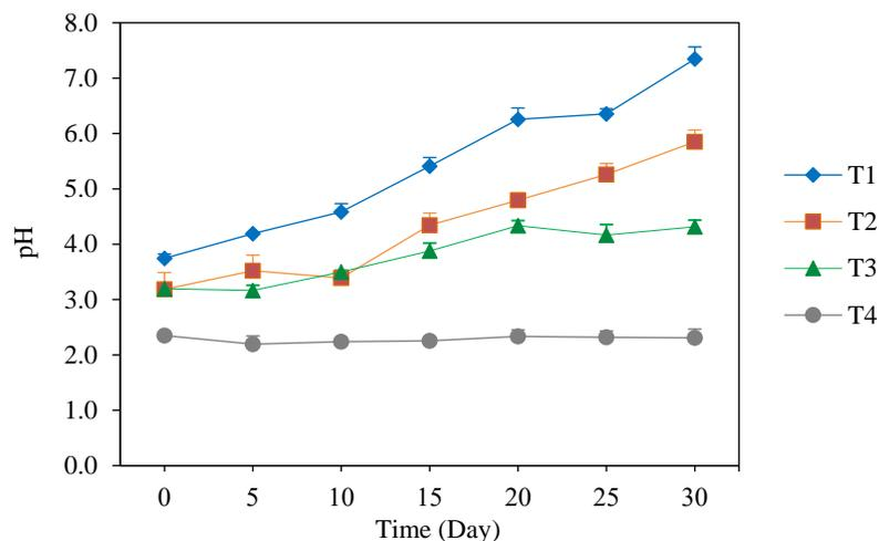
**Figure 5.** Changes of pH in acid mine water with treatments: 10% sediment and 5% compost (T1), 10% sediment (T2), 5% compost (T3) and without added sediment and compost (T4)
