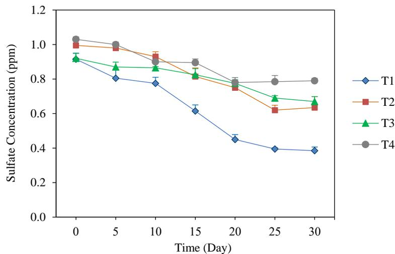
**Figure 4.** Sulfate concentration in acid mine water with treatments: 10% sediment and 5% compost (T1), 10% sediment (T2), 5% compost (T3) and without added sediment and compost (T4)
