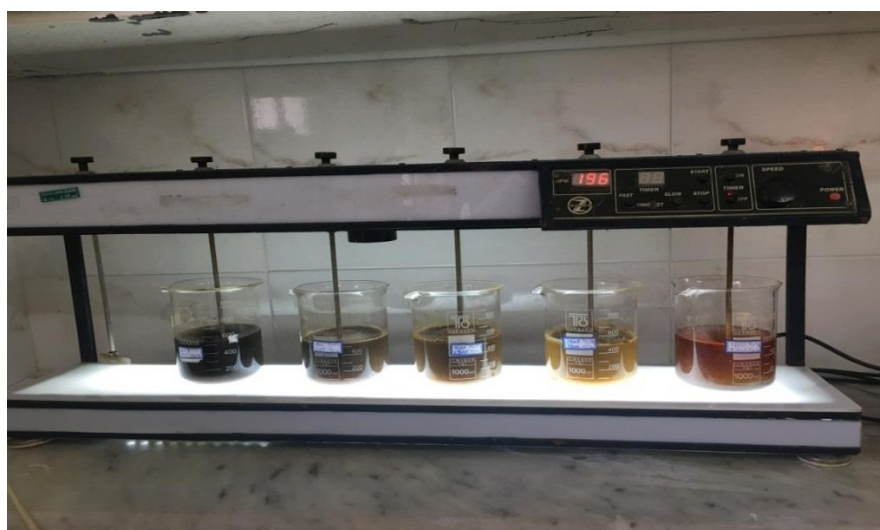
Figure 2. The study of the Fenton process in the jar test at different ratios of \text{H}_2\text{O}_2/\text{Fe}^{+2}
