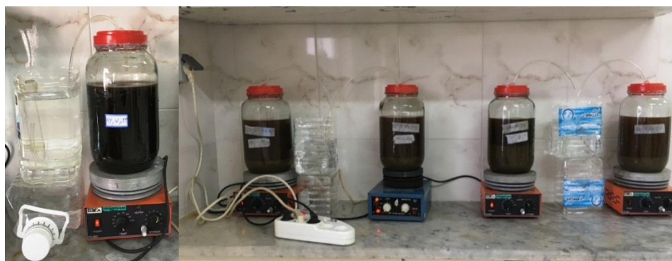
Figure 1. The primary reactors with retention times of 5-25 days
