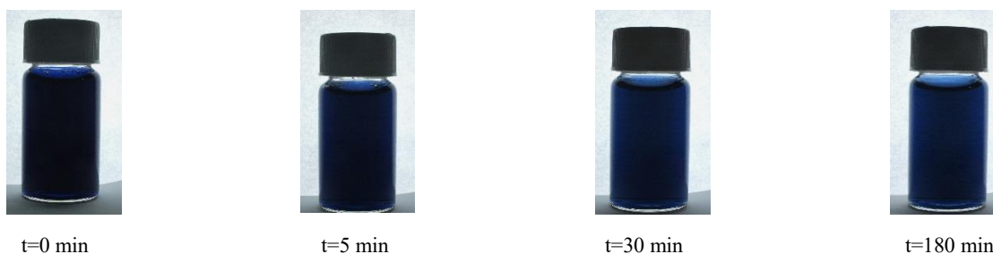
Figure 12. Change in color during MB dye degradation in absence of NaBH 4 .
