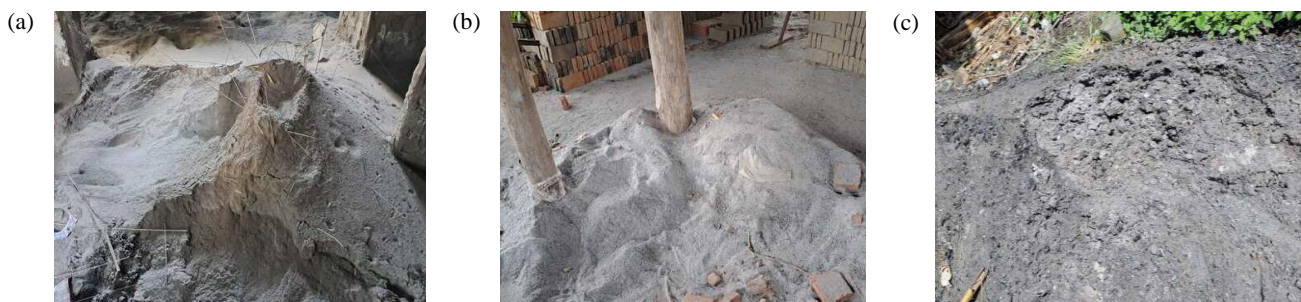
Figure 1. Types of agricultural ashes (a) sugarcane bagasse ash, (b) rice husk ash, (c) coir-wood ash
