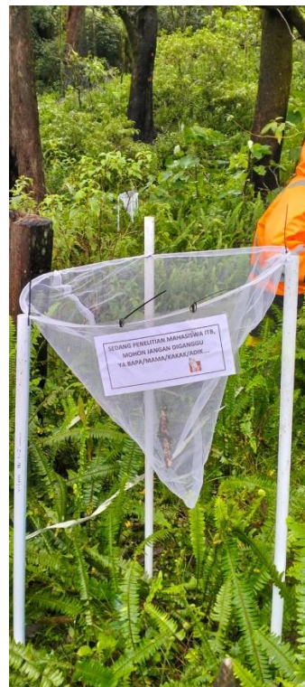
Figure 2. The setup of the seed trap at the study site
