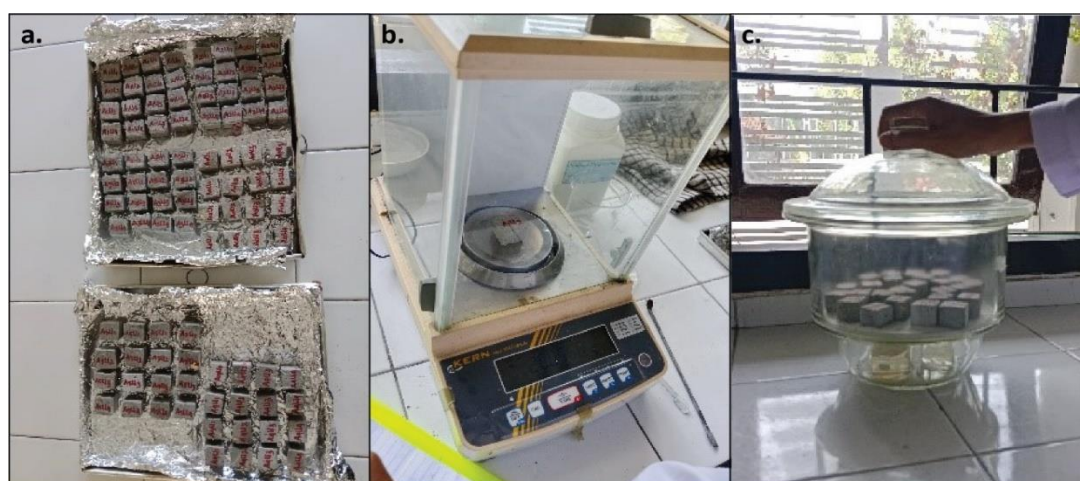
Figure 5. Pollutant adsorption test: a. Mortar cube; b. Sample weight; c. Pollutant induction in desiccator
