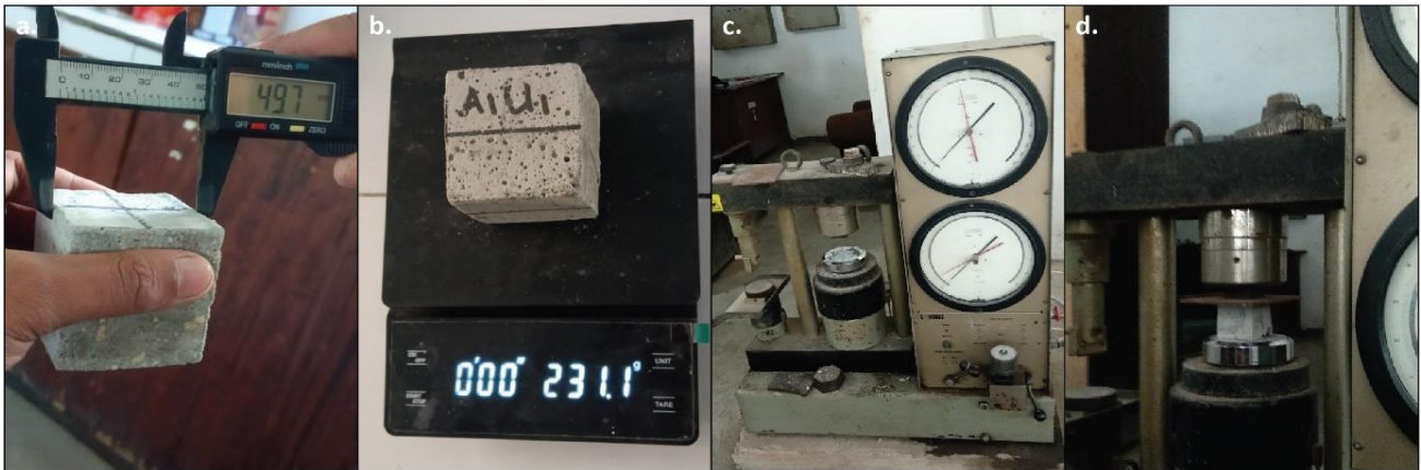
Figure 3. Test specimen; a. mortar cube; b. sample weight; c. and compressive test; d.
