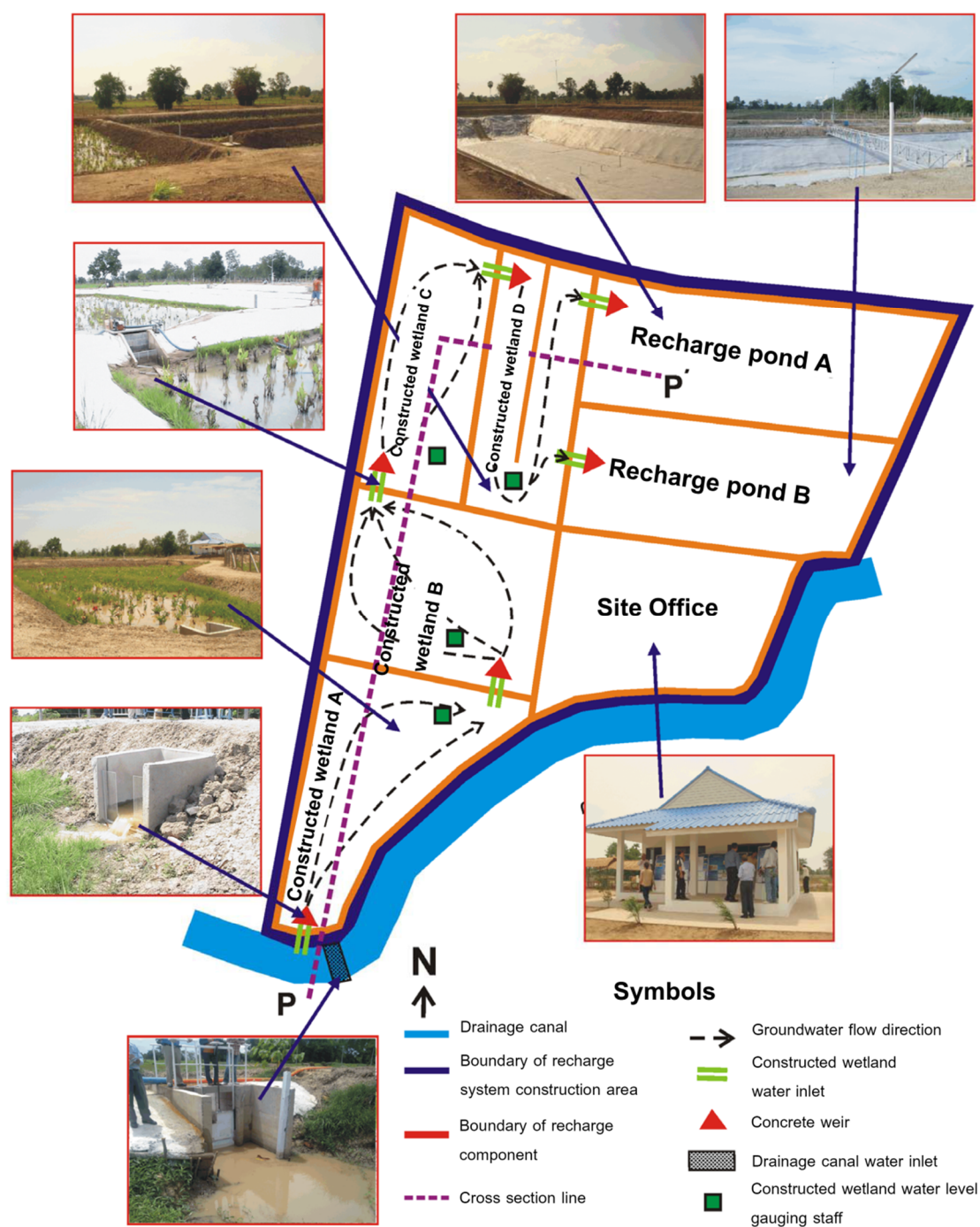
Figure 4 Components of the ponding system including four constructed wetlands for pretreatment and two recharge basins (Department of Groundwater Resources, 2011)
