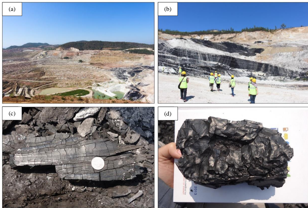
Figure 2. (a) Mae Than open-pit coal mine (looking west), (b) coal seams and Inter Burden sediments (looking north), (c) woody texture coal, and (d) hard bright coal
