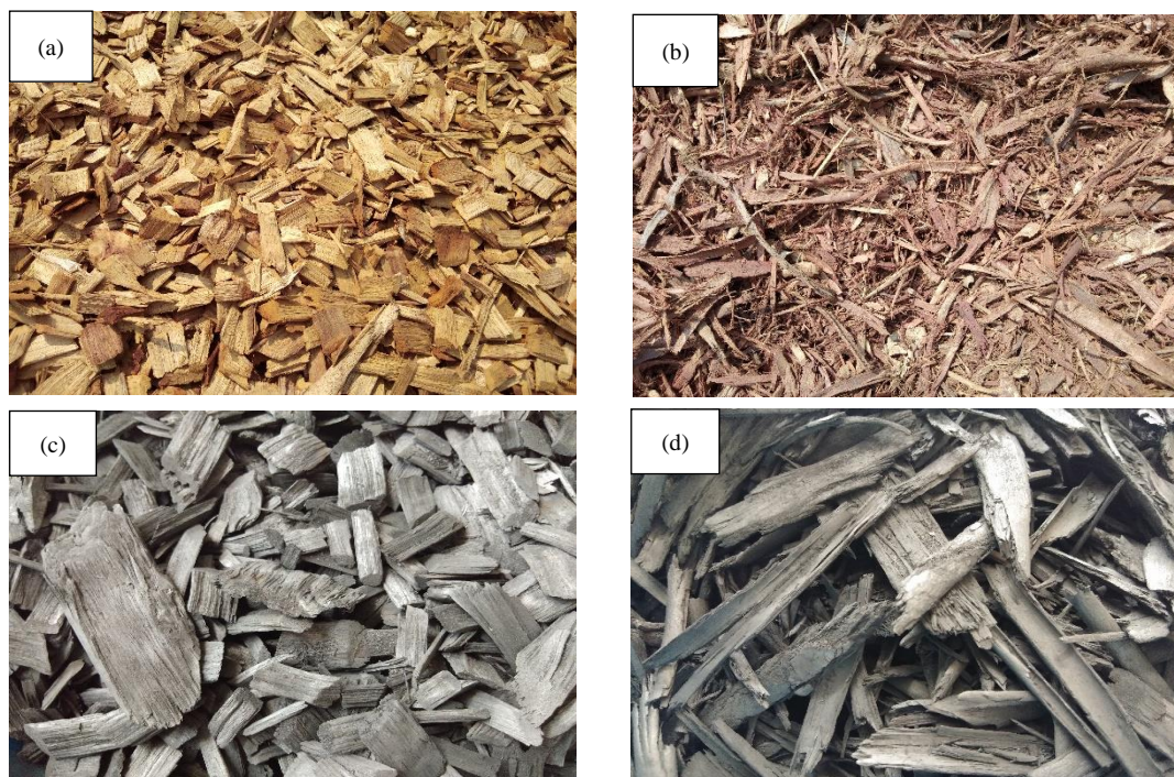
Figure 1. Physical structure: eucalyptus wood chips (a); eucalyptus bark (b); eucalyptus wood chips after carbonization (c); and eucalyptus bark after carbonization (d)
