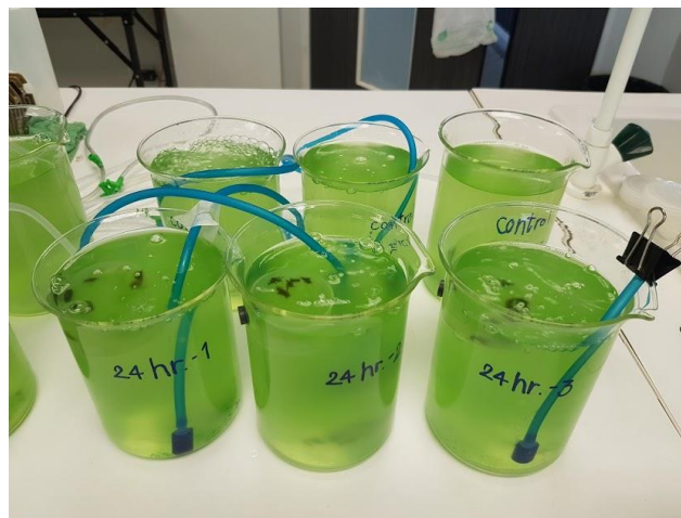
Figure 4. Experimental setup to investigate wastewater treatment efficiency by bryozoans
