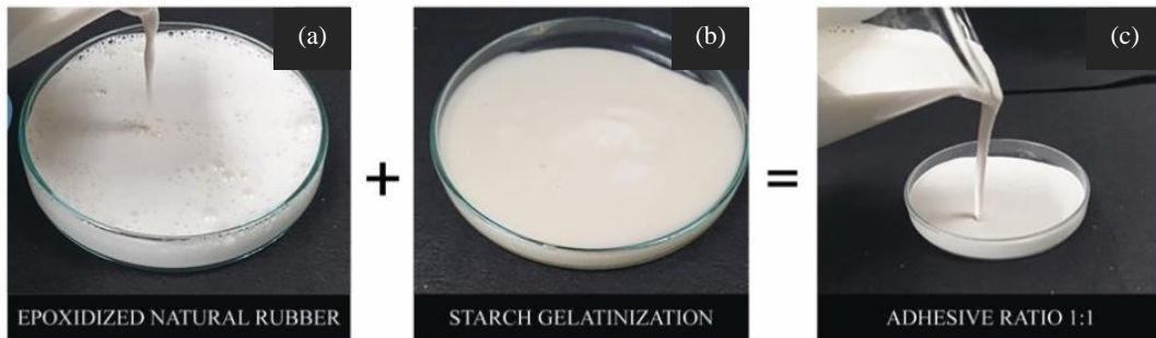
Figure 2. (a) ENR (b) GTS and (c) Adhesive (1:1 weight ratio)
