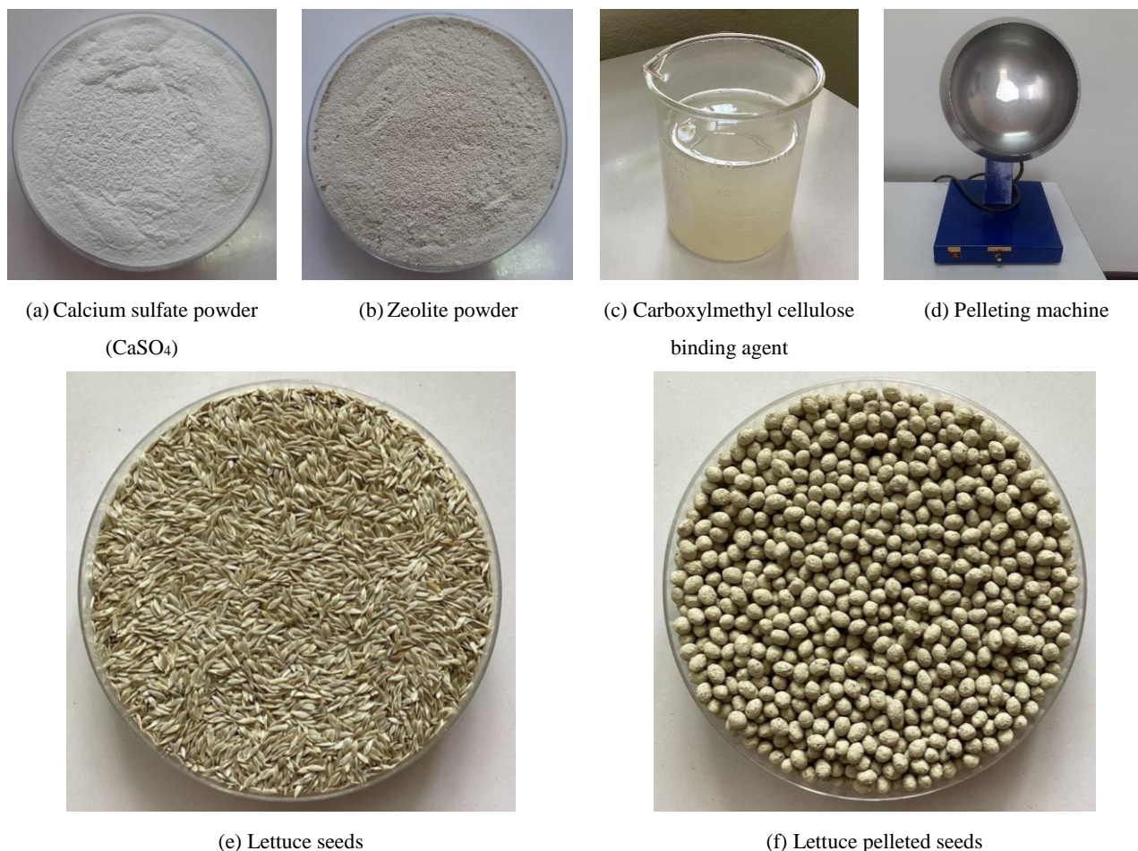
Figure 1. Characteristic of filler types (a-b), binder type (c), pelleting machine (d), Lettuce seeds (e), and Lettuce pelleted seeds (f)
