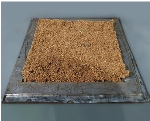
Figure 1. A 30×30×0.5 cm square mold with a mixture of coconut shell particles and the adhesive
