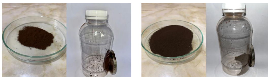
Figure 7. Sample adsorbents of (a) magnetic biochar and (b) layered double hydroxide Zn-Al/magnetic biochar composite
