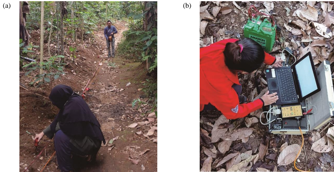
Figure 2. Seismic refraction measurement: (a) one of seismic trajectories, and (b) measurement tools Doremi 24 channels
