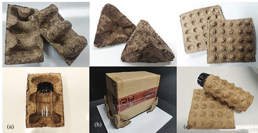
Figure 6. Three forms of final cushion packaging: (a) bottle type, (b) corner type, and (c) wrapping type
