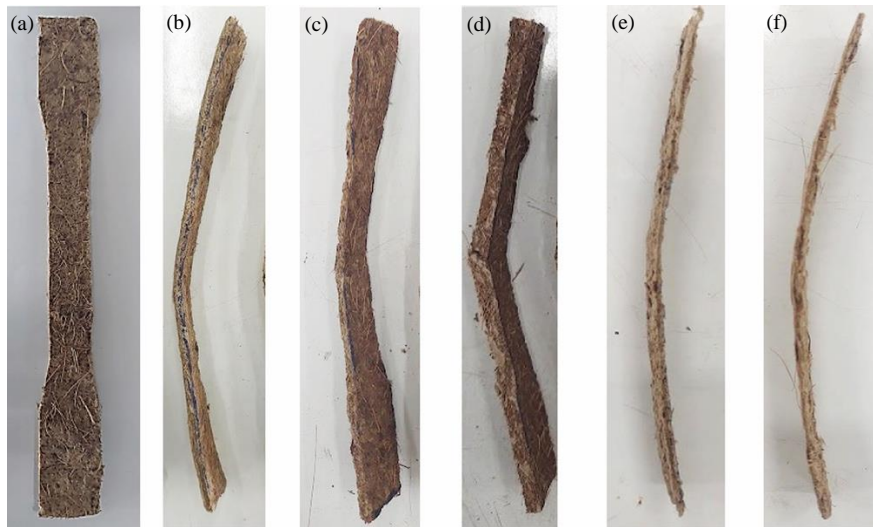
Figure 4. Flexural test results of paper, untreated coconut fiber, and coconut coir dust at various ratios: (a) shape before testing, (b) 60:20:20, (c) 40:20:40, (d) 20:20:60, (e) 80:20:0, and (f) 60:40:0
