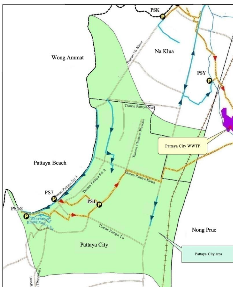
Figure 5. Wastewater collection system for Pattaya City WWTP
