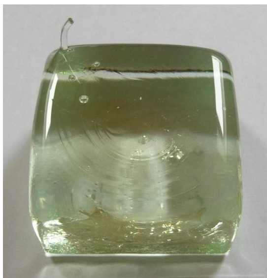
Figure 6. Molten glass sample (40×40×20 mm) from Brunei silica sand
