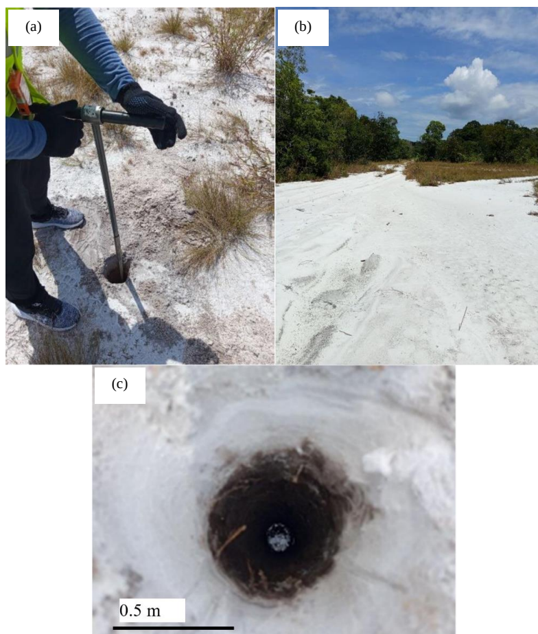
Figure 3. (a) Coring with auger (b) Surrounding environment at site 1 (c) Reflection of the groundwater table at borehole 3 (BH3)
