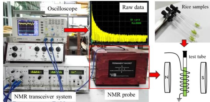
**Figure 1** The experimental setup with TeachSpin's Pulsed NMR
