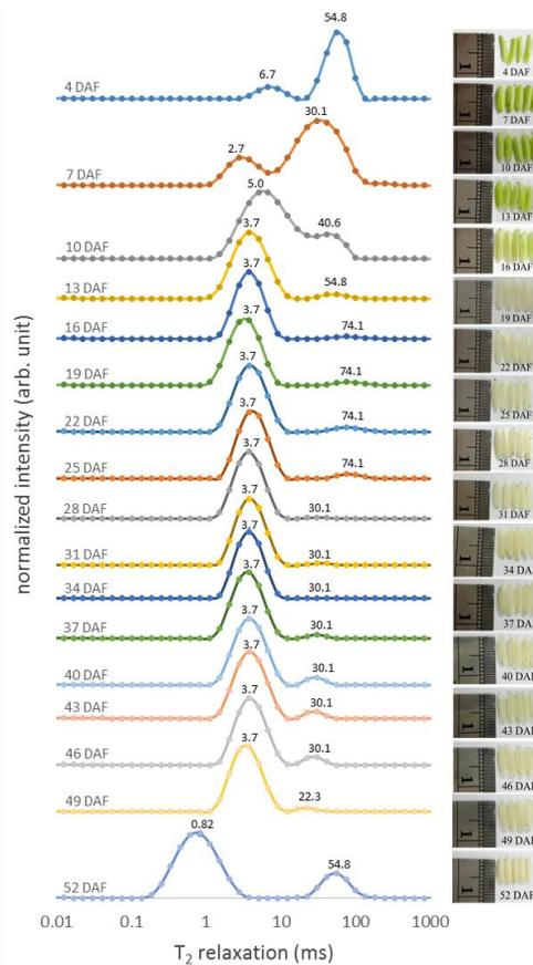
**Figure 4**  $T_2$  relaxation times distribution curves of Thai rice kernels at different grain stage
