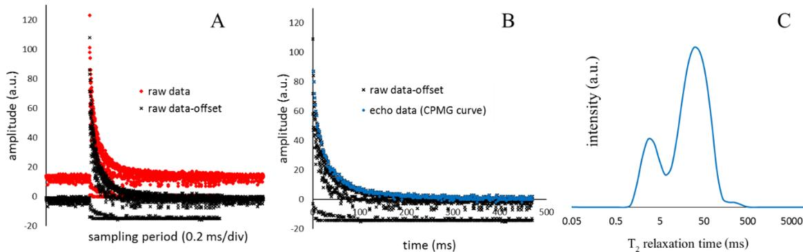
**Figure 2** (A) Raw data before and after eliminating the noise backgrounds, (B) the raw data without the noise and the echo data as a function of the echo time, and (C) the distribution of  $T_2$  relaxation time obtained using ILT
