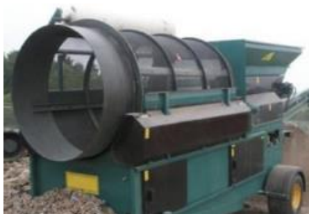
Figure 1 Illustration of a Revolving Screen or Trommel.
