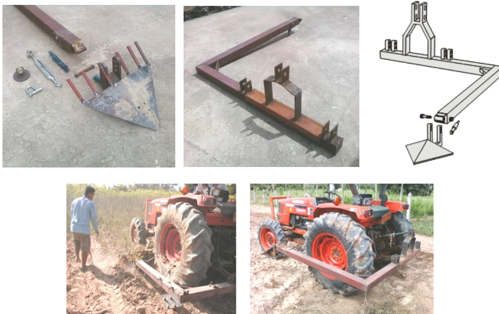
Figure 2 Components of the experimented cassava digger attached to the tractor's side
