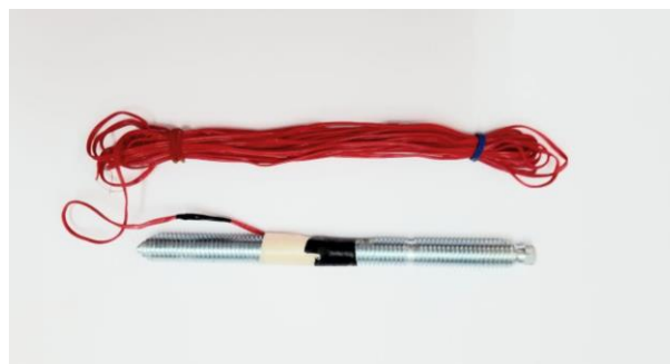
Figure 14 Strain gage attached on shear bolts
