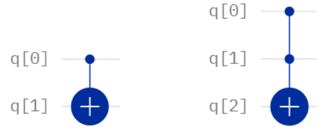
(a) The CNOT gate (b) The CCNOT gate
