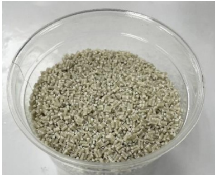
Figure 3: Granule of short glass fiber/ABS composites.
